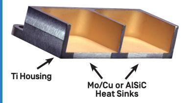
aluminum and can remain hermetic with walls as thin as .010". This means an existing aluminum package can be redesigned to be stiffer, lighter weight, more reliable, and better thermally, by integrating PA&E's titanium composite technology. Titanium is compatible with both resistance and laser welding processes for flexibility in connector integration and cover sealing.
