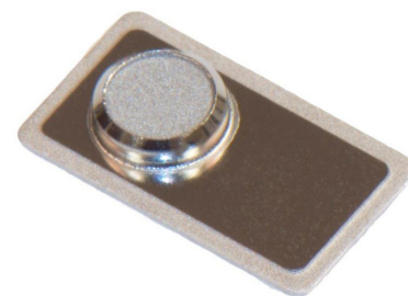
Getter assembly as typically supplied. In this case the getter housing is attached to a stepped lid. This integrates the getter into the device at the point of lid sealing.
