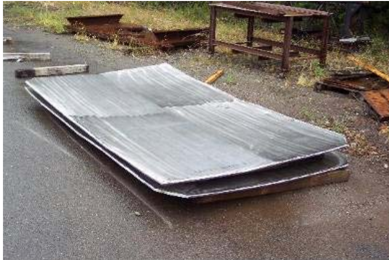
Ni/Inconel plates before flattening
