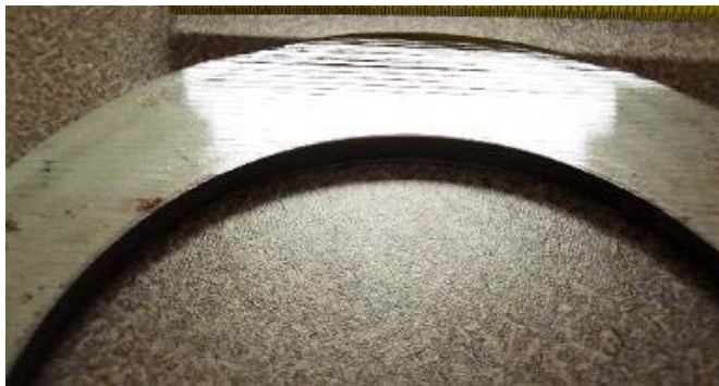
Tantalum on I.D. of steel pipe
