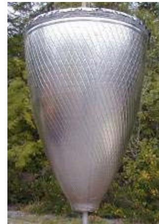
Space Shuttle Cone and After Explosive Forming
